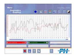
Six channels are available. It enables to plot from one to six signals simultaneously with a sampling frequency from 2 to 10 Hz.
