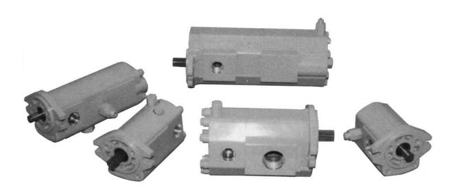
PRINCE SP PUMPS WITH INTEGRAL VALVING FEATURE EXTRUDED ALUMINUM REAR COVERS. THE EXTRUDED REAR COVERS ALLOW EXCEPTIONAL FLEXIBILITY FOR INCORPORATING DIFFERENT VALVING AND PORTING OPTIONS. PRINCE'S USE OF COMPUTER CONTROLLED MACHINING CENTERS IN THE MANUFACTURING PROCESS ALLOW EITHER STANDARD OR CUSTOM DESIGNS TO BE MADE IN BOTH SMALL AND LARGE QUANTITIES.
