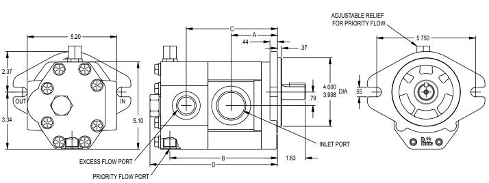
RIGHT HAND ROTATION SHOWN. FOR LEFT HAND ROTATION, INLET AND EXCESS FLOW PORTS GO TO THE OPPOSITE SIDE OF THE PUMP, PRIORITY FLOW PORT GOES FROM THE BOTTOM TO THE TOP OF THE PUMP.
